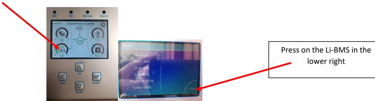
You should see three lines of info for the NV14 and five lines of info for the NV24. This assures that the batteries are communicating. If this information is not correct, then try resetting the communications cables into the batteries.
